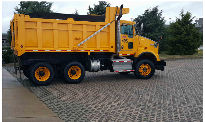
Photograph PPS-4. CGP installation allows for infiltration into subsurface via permeable infill material. Photo: True Grid.
