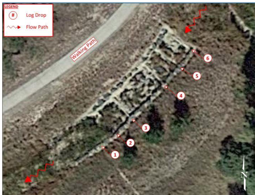
Figure 2: Drop Structure Locations
