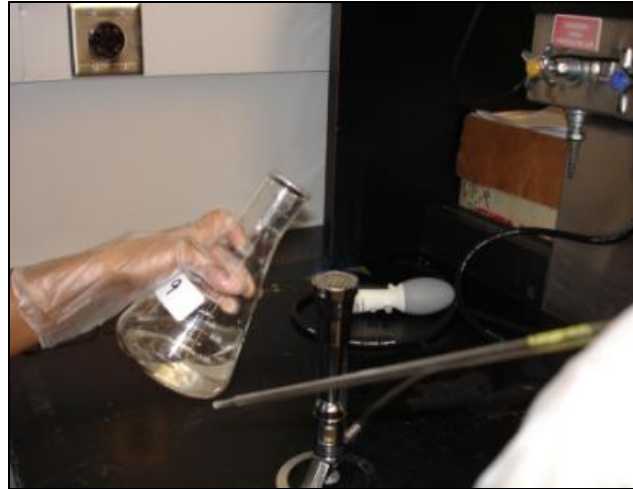
Microcosm in an Erlenmeyer flask being pipetted for FIB analysis using sterile techniques. (Photo Courtesy of Dr. Cristiane Surbeck, University of Mississippi)
