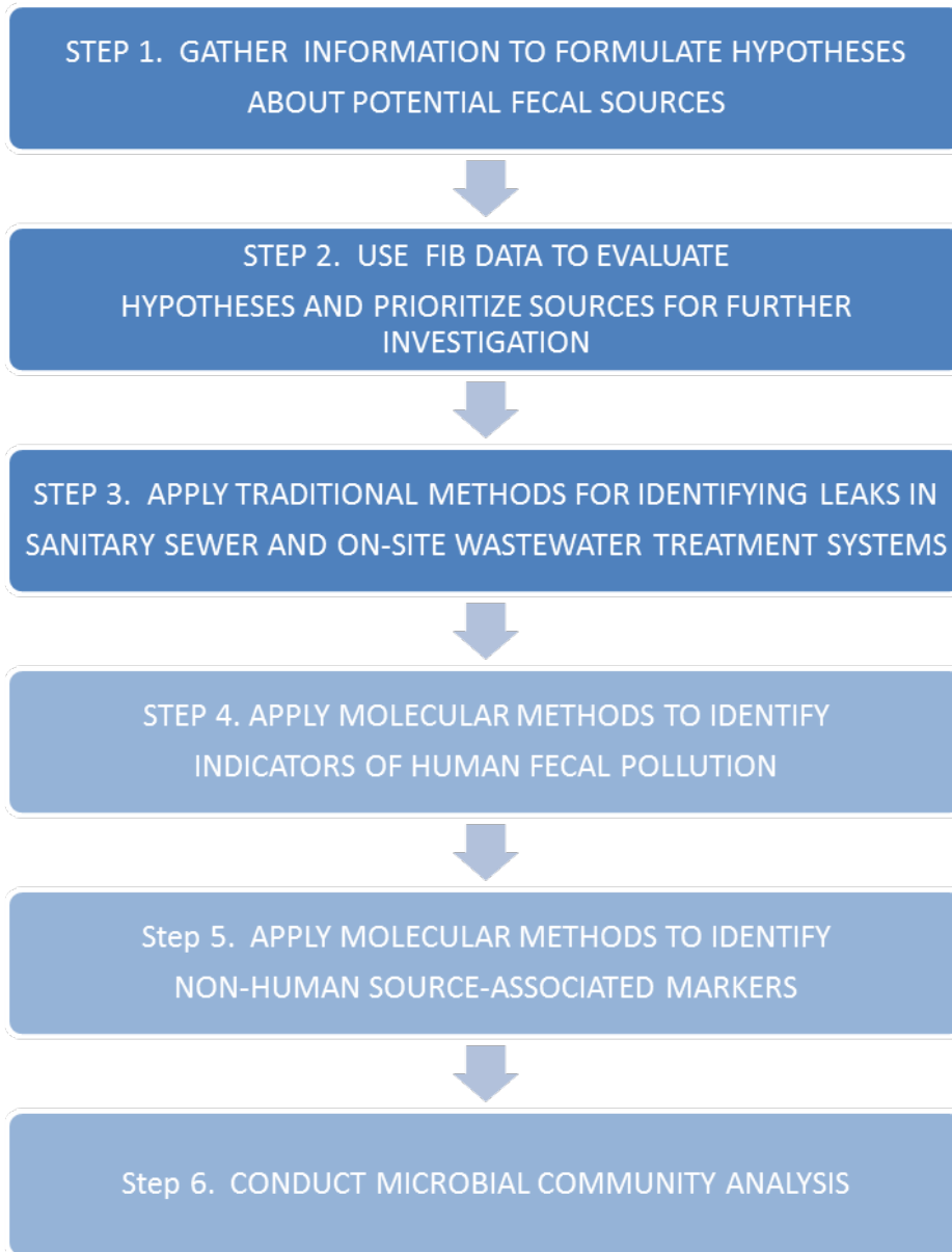
Figure 5-1. Six-Step Process of Microbial Source Identification (Based on Recommendations in Griffith et al. 2013)
