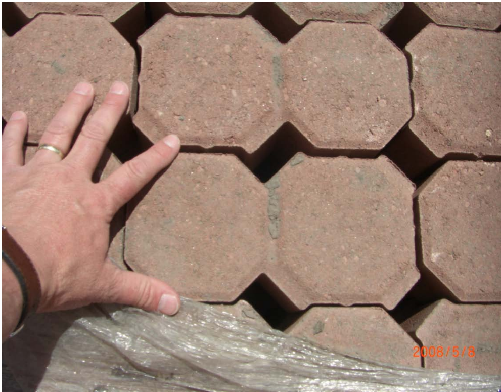
Photograph 3. Concrete block pavers prior to placement.
