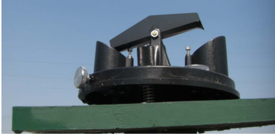
Photograph 4. The tipping bucket of the rain gauge assembly (cover and funnel assembly removed)
