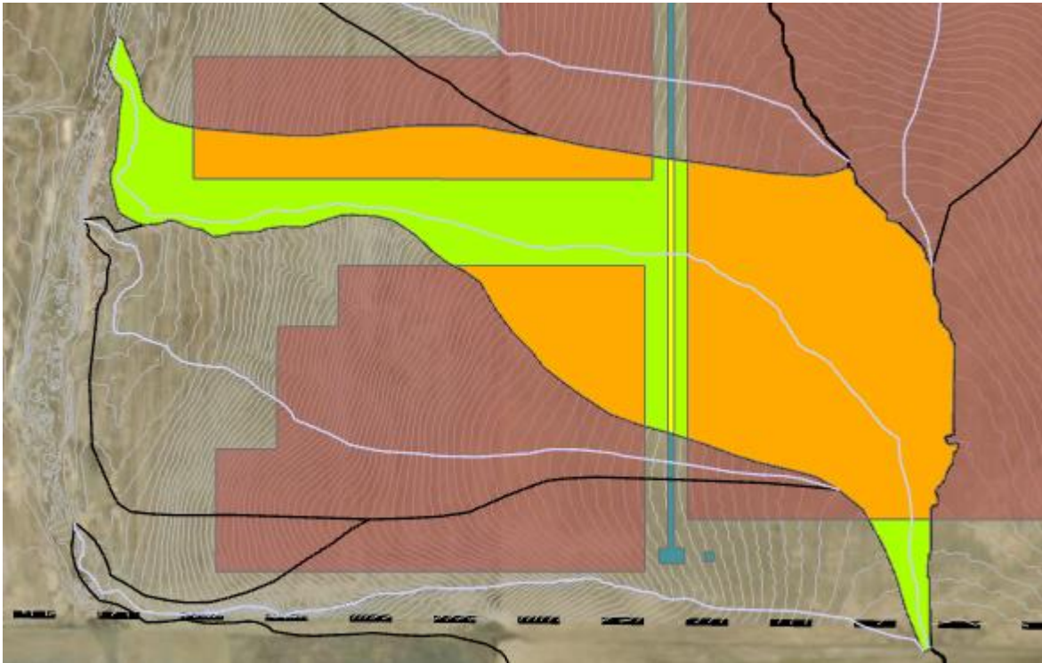
Figure EX-3. Land Cover Categories in Sub-basin 5 Include Open-space (Green), Solar Panels (Orange), and Gravel (Yellow)
