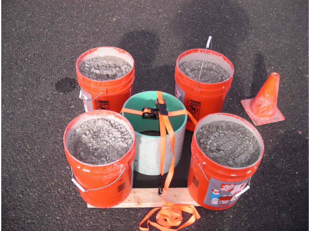
Photograph 7. The apparatus used for the infiltration test on December 9, 2010.
