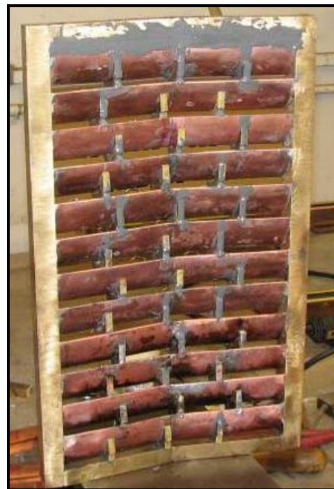
Figure 3-7: Type 16 grate during fabrication
