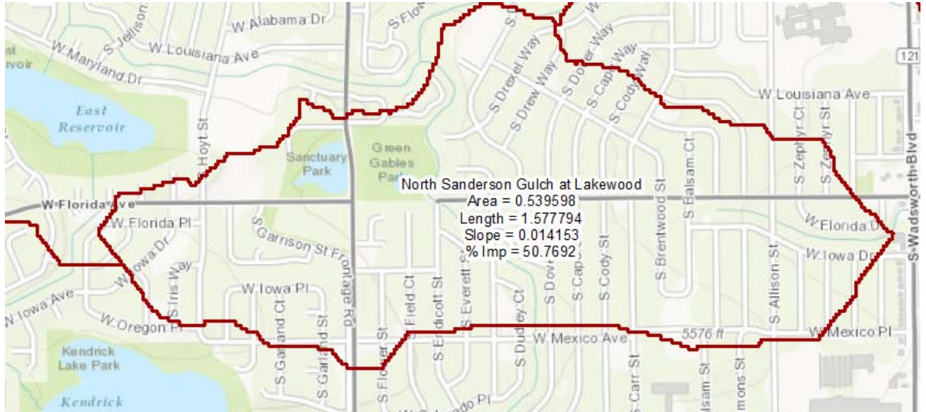
Figure 16 - Sanderson Gulch at Lakewood Upstream of Wadsworth
