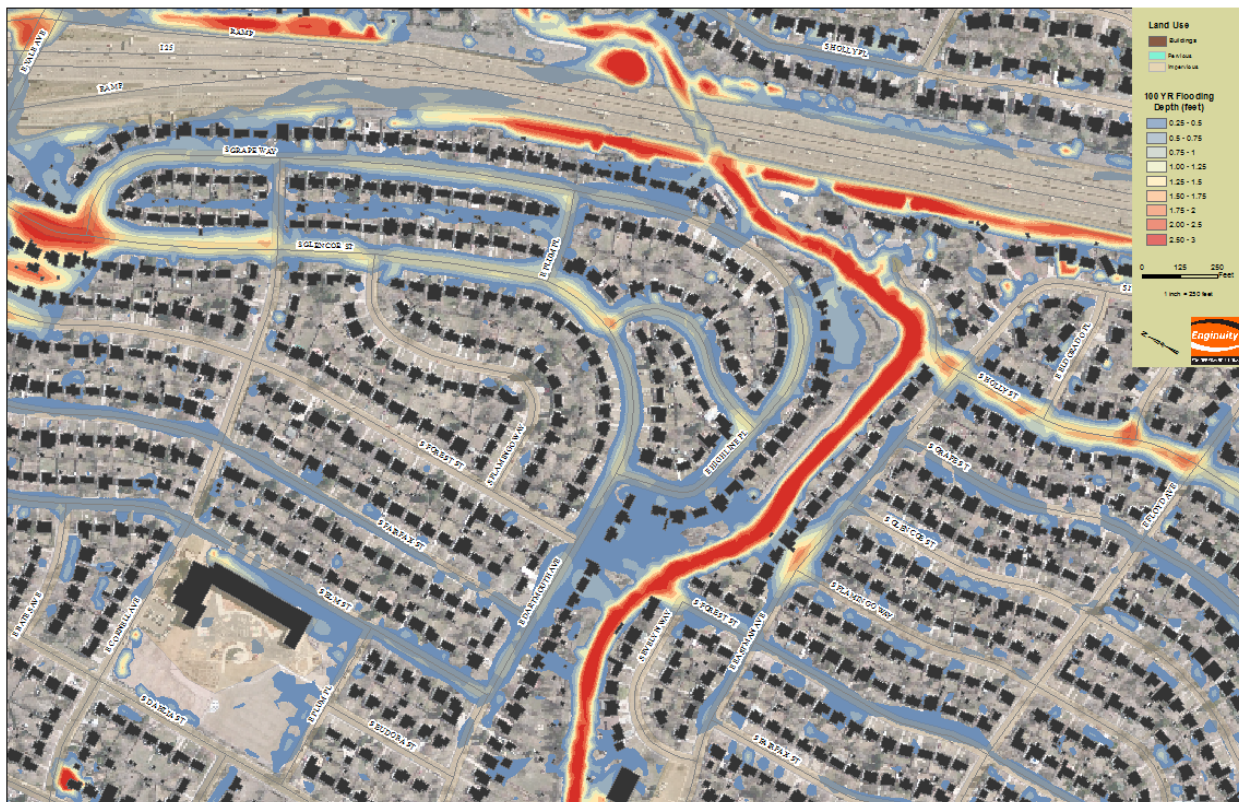
Figure 7 - Image of 2D Rain on Grid Model of Upper Harvard Gulch at the Highline Canal
