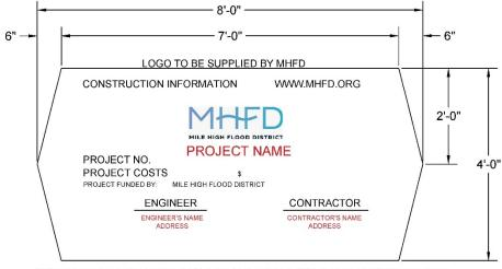
SIGN TO BE ON 3/4" MARINE PLYWOOD AND HAVE A SKY BLUE BACKGROUND WITH BLACK LETTERING. EMBOLDED LETTERS AND 3" HIGH, ALL OTHERS ARE 2" HIGH. POSTS SHALL BE 4" X 4" CEDAR WOOD. SIGN SHALL BE ATTACHED TO POSTS WITH (4)-1/2" X 3" LAG BOLTS.
