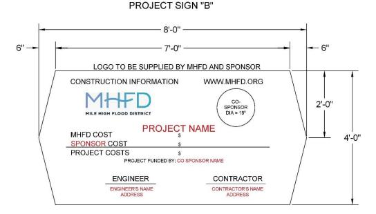
SIGN TO BE ON 3/4" MARINE PLYWOOD AND HAVE A SKY BLUE BACKGROUND WITH BLACK LETTERING. EMBOLDED LETTERS AND 3" HIGH, ALL OTHERS ARE 2" HIGH. POSTS SHALL BE 4" X 4" CEDAR WOOD. SIGN SHALL BE ATTACHED TO POSTS WITH (4)-1/2" X 3" LAG BOLTS.
