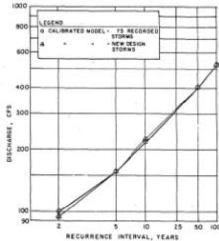
Figure 13. Peak Flow Distribution Using New Design Storms for Englewood Site
