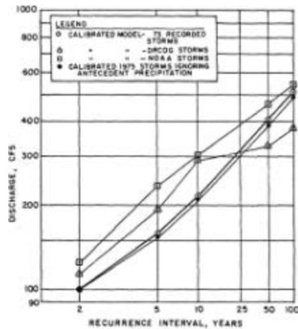
Figure 9. Peak Flow Probability Distribution for Englewood Site
