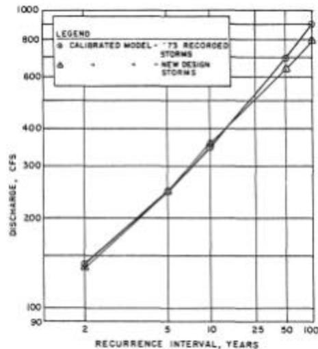
Figure 11. Peak Flow Distribution Using New Design Storms for Northglenn Site
