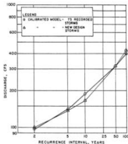
Figure 12. Peak Flow Distribution Using New Design Storms for Denver Site
