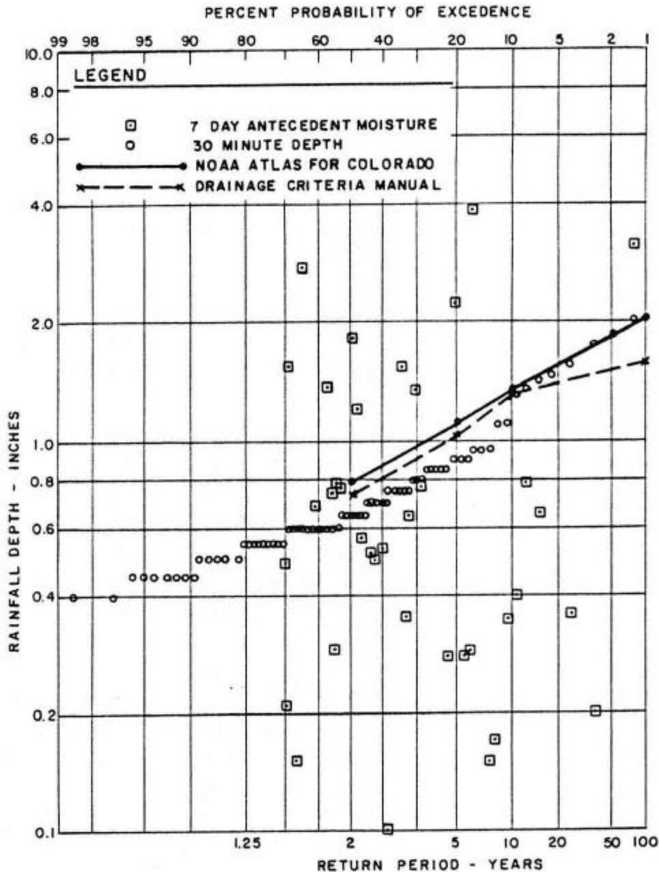
Figure 1. Probability Distribution Of 30-Minute Rainfall Depths at Denver Raingauge, 1898 through 1971.
