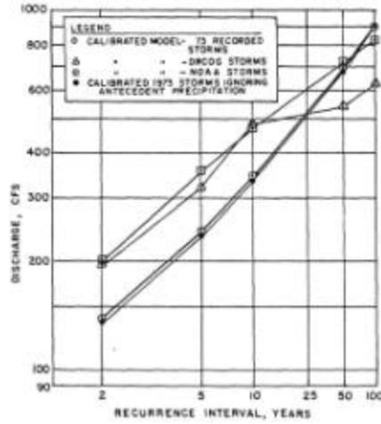
Figure 7. Peak Flow Probability Distribution for Northglenn Site
