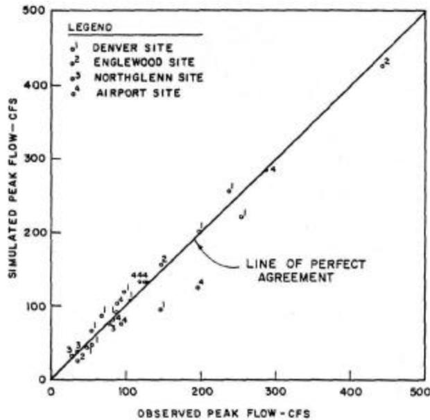
Figure 6. Comparison of Simulated and Observed Peak Flows
