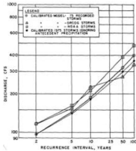
Figure 8. Peak Flow Probability Distribution for Denver Site
