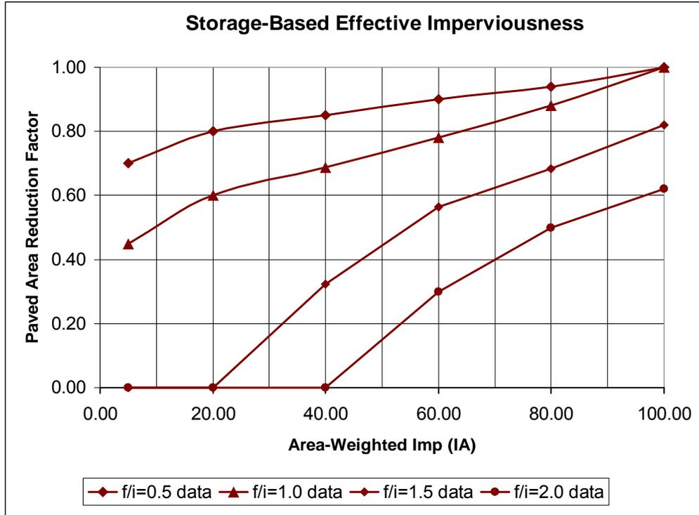
**Figure 3 Storage-Based Pavement Area Reduction Factor**
