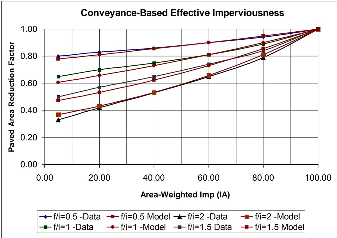
**Figure 2 Conveyance-based Pavement Area Reduction Factor**
