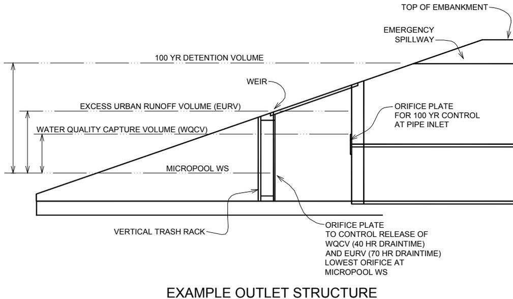
Figure 5. Typical outlet structure conceptual profile for modeling *full-spectrum detention*. For details of this outlet download Ref. UDFCD (1992 & 1999)
