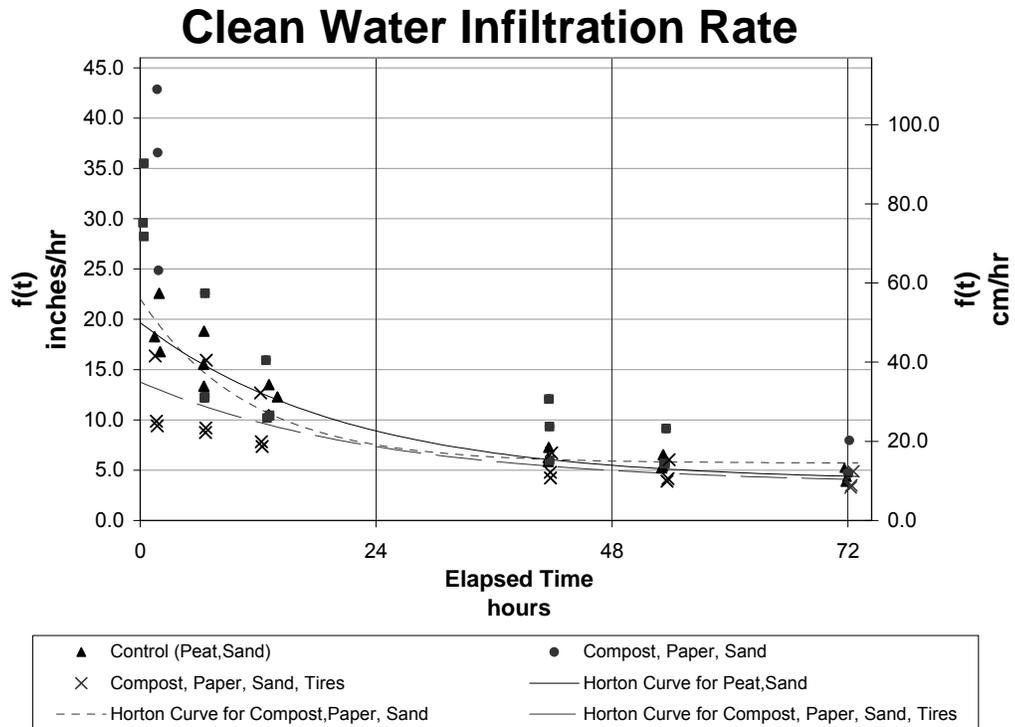
**Figure 10 Infiltration Rate**
