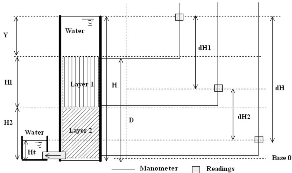
**Figure 8 Illustration of Infiltrometer Operation**
