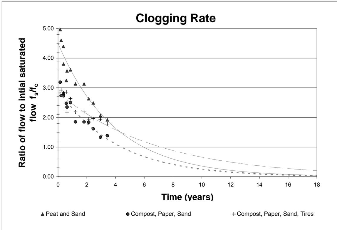
**Figure 12 Reduction of Infiltration Rate for Example PLD**
