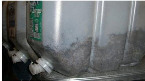
**Figure 4 Batch Test Set-up for Collection of Leachate and Flow Rate**
