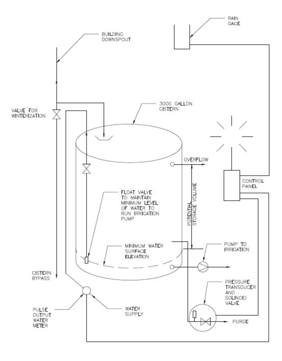
Figure 1. DGS rainwater harvesting schematic.
