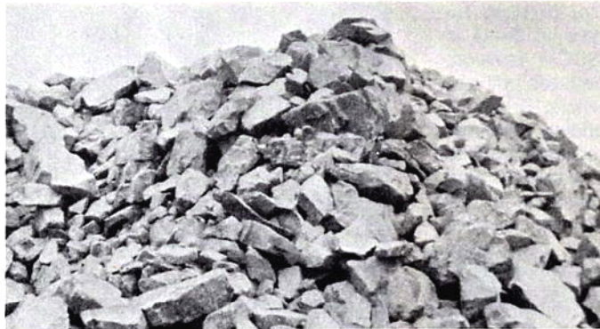
Figure 5 - A stock pile of Medium (M) riprap. Note the variation in the size of the rock.
