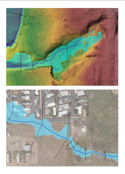
1. Contraction and expansion coefficients are not placed where flow velocities increase or decrease significantly. In general, for bridge and culvert modeling, the coefficients should be increased at two upstream cross sections and one downstream cross section.
