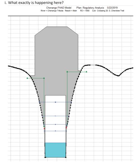
**Response:** The bridge deck has been modified by hand to reflect obstruction of flow that would be caused by the large chain-link fence located along the headwall of the culvert. The road crest is actually lower than the headwall elevation at this location, so embankment blockage is only represented by the headwall and chain-link fencing.
