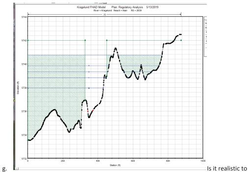
force all the flow to remain north of the road and flow into the culvert? The topo (as well as the lack of any defined channel downstream of Parker Rd.) suggest this is not what happens.
