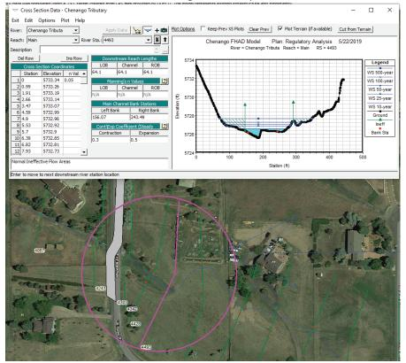
Response: Expansion/ contraction coefficients were generally applied along the full distance that contraction took place upstream of structures. The coefficients have been limited to the two XS's upstream instead of three.
