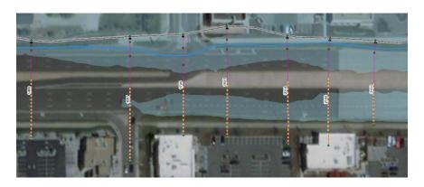
**Response:** It is believed that flow does make it over to the south side of Arapahoe via the upstream split. It does not appear to recombine with the "main channel" on the north side of Arapahoe, and therefore was modeled as ineffective flow.
