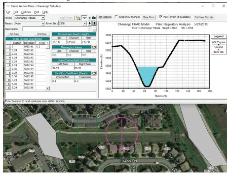
Response: The channel CL is delineated to follow the contours for low flow, while the overbanks are following a less-sinuous overbank flow path. While the channel reach length is slightly longer than the overbanks, all three will be averaged out in the calculations.
