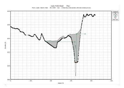
**Response:** Modified culvert inverts/ground elevations to match survey.
