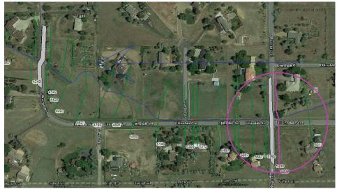
Response: SWMM flow change locations were offset upstream to the next SWMM design point. When the design point was located at a road crossing, the flow change was applied at the structure's downstream XS so that the "correct" flow was applied through the structure. Confirmed this is okay at meeting.
