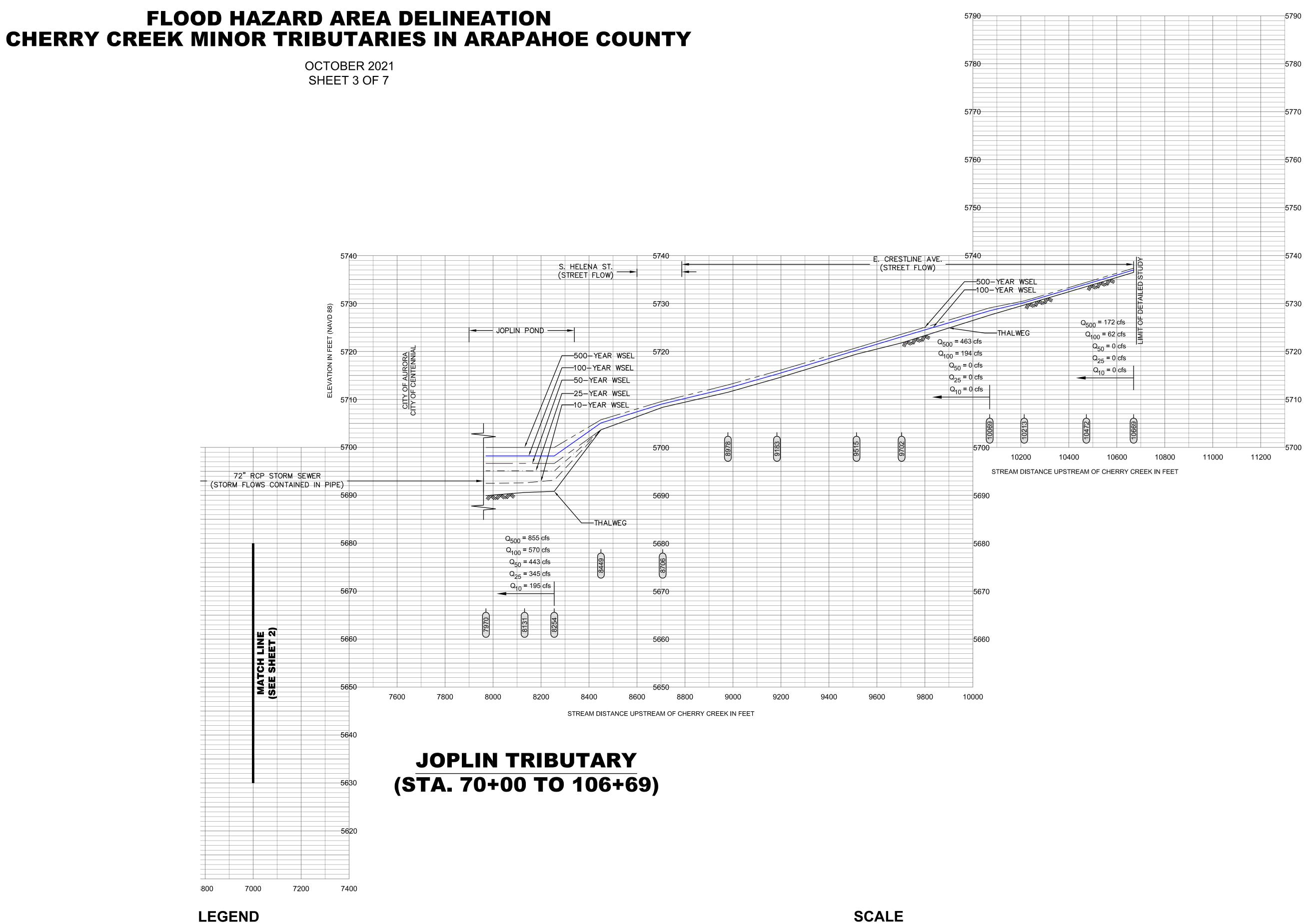
500-YEAR WATER SURFACE ELEVATION **100-YEAR WATER SURFACE ELEVATION 50-YEAR WATER SURFACE ELEVATION** 25-YEAR WATER SURFACE ELEVATION **10-YEAR WATER SURFACE ELEVATION** \_\_\_\_\_ — STREAM BED
