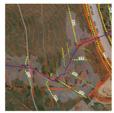
a. The skew of these XSs in the overbank seems as though it doesn't always accurately represent the actual flow direction of water and requires big differences in overbank and channel reach lengths. Please explain the reasoning for these alignments.
