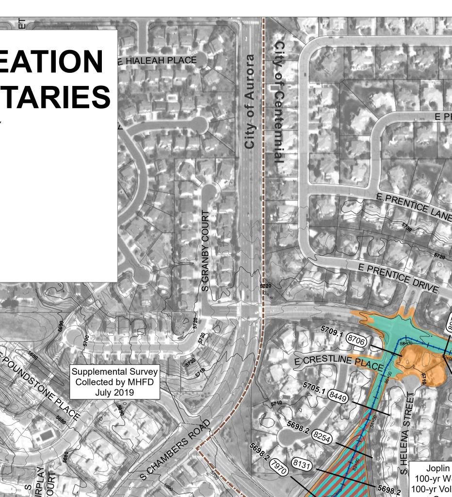
$Q_{100,in} = 570 \text{ cfs}$  $Q_{100,out} = 352 \text{ cfs}$
