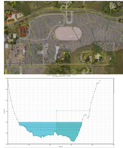
Response: 3955 to 2419: IEFA on right raised to eliminate other possible flow channel and reflet ineffective flow spilling out into park. The other channel has a longer flowpath and when crosssections are cut for our delineated channel, a straight-line runs through the opposing channel at a point when it's lower (for approx. two XSs). It should remain IEFA because downstream near Parker Rd., the flow pools and slinks back to the ditch, which is the main low-flow channel we are following.
