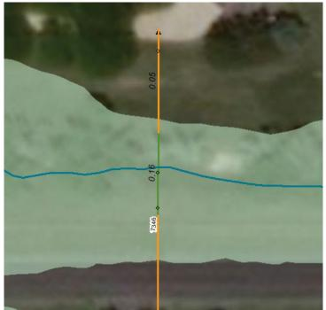
**Response:** Bank stations corrected per modification of XS stationing to start at 0.
