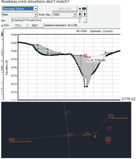
Response: Road deck elevations have been modified by hand to correspond with the structure survey.
