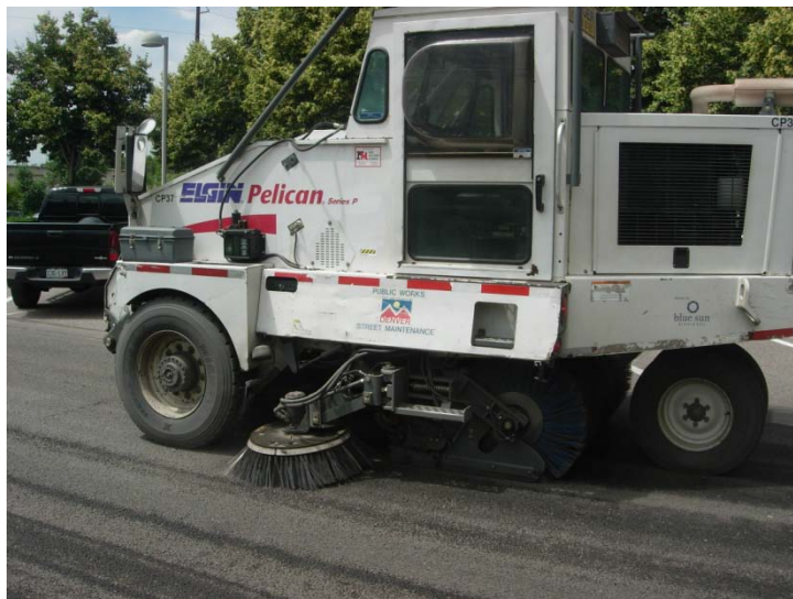
Photograph 6-4. This broom sweeper will only remove debris from the pavement surface. Broom sweepers are not designed to remove solids from the void space of a permeable pavement. Use a vacuum or regenerative air sweeper to help maintain or restore infiltration through the wearing course.
